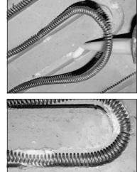
bedding the element in Pyrolite could cause the element overheat.
