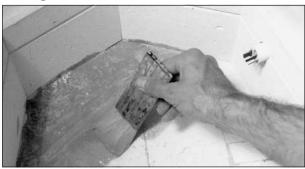
Coat the firebrick floor with kiln wash or glass separator. If your kiln has sidewall elements, hold a piece of cardboard in front of the elements to protect them from contact with kiln wash.
