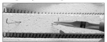
brick better than pressing the staples straight in.) Press the staples until flush with the surface of the firebrick. Be careful to avoid pressing a staple into an element. The staple should also be short enough so that it does not touch the kiln case on the other side of the brick wall.
