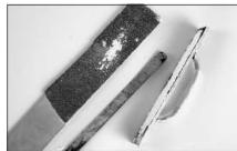
The left sanding block is 1 ¼" wide; the right sanding block is 1" wide. In the center is a hack-saw blade used to cut firebricks.
