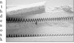
two staples tilted away from each other. (Pressing the staples in at an angle holds the broken
