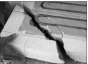
The ideal way to cement bricks together is along flat surfaces, because sliding the surfaces together after applying the cement makes a thin seam.
