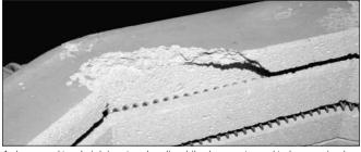
A damaged top brick in a top-loading kiln does not need to be repaired so long as 1  $\frac{1}{2}$ " of brick surface remains to form a seal against the lid. The brick still supports the element.
